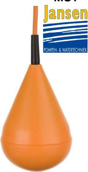
The MS 1 level regulator is a single-point regulator, specially designed for use in wastewater treatment plants and in pump stations which handle liquids polluted with solids. Thanks to its good chemical properties, it is resistant to a wide range of liquids.
